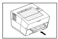
Adjust the paper width guides and slide the paper into the tray as far as it will go. The side to be printed should be face up.
